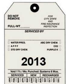
Typical service company annual maintenance tag
